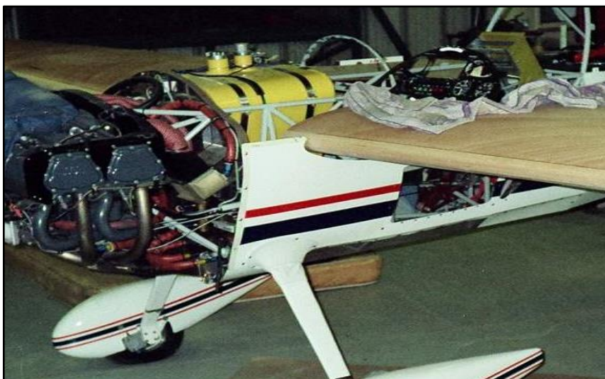
Photo No. 2: The fuel tank (painted yellow) as seen during aircraft construction.
